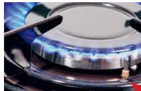
Gas cooker with safety pilot The red arrow indicates the thermocouple
